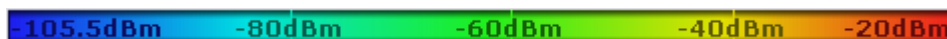
Fig. 3-48: Linear color curve shape = 0; colors are distributed evenly over the complete result range
